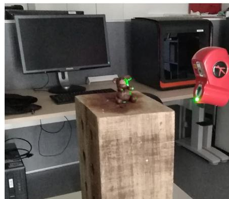
^ A Kreon Scanner was used for scanning the polymer clay bears.
